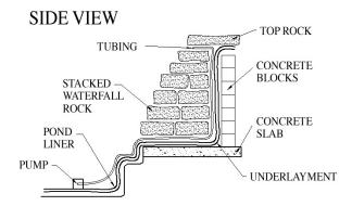
Fold the liner up and over the top layer of rock. Lay your waterfall rock over the tubing and liner to conceal it. Plug in the pump and test your waterfall.
